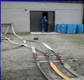
Test Header with Flow Meter Setup
