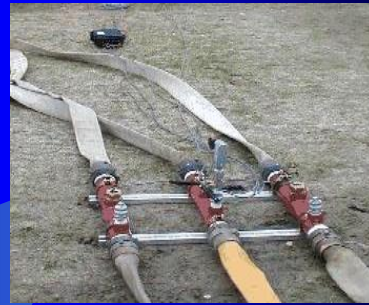
Flow meters measure system flow and conductivity sensor (center) measures injection rate
