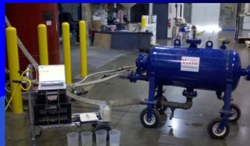
Planit Safe™ liquid interface tank connected to foam system
