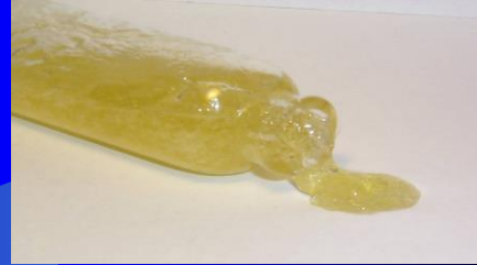
Substitute liquid mimics the physical properties of foam concentrate (Even viscous AR-AFFF types)
