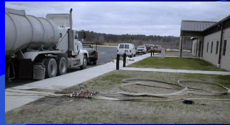
Typical test setup with tanker for collection and disposal of foam
